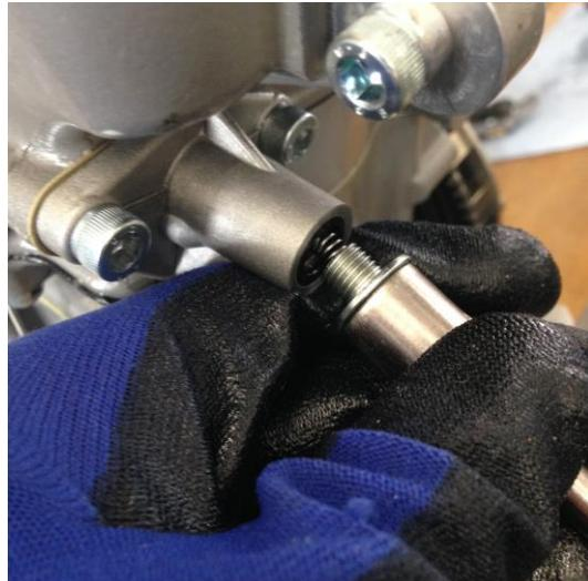
Place the spring in the automatic cam chain tensioner and tighten it. Always check if the o-ring is still on!
