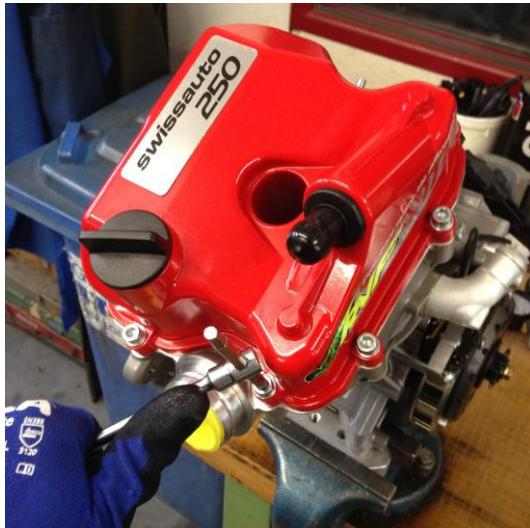
Remove the cam-cover (8 M6 bolts).
