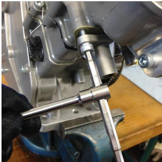
Disassemble the automatic cam chain spanner (2 bolts).
