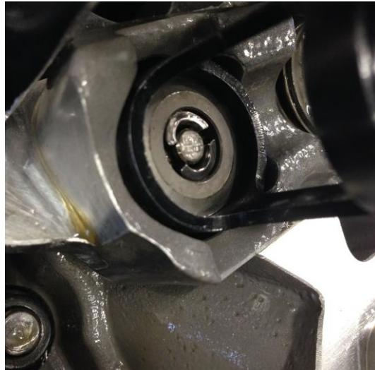
Hang the press unit under the bridge of the camshaft compressing tool and slowly increase the pressure on the top of the valve retainer by turning in the compressing tool.
