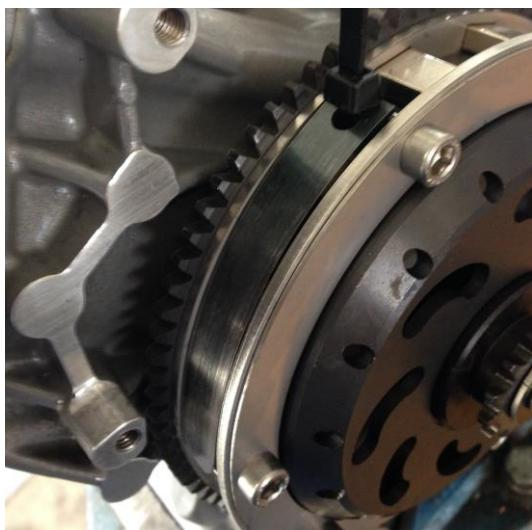
The tool must be positioned between the attachments for the charge coil.
