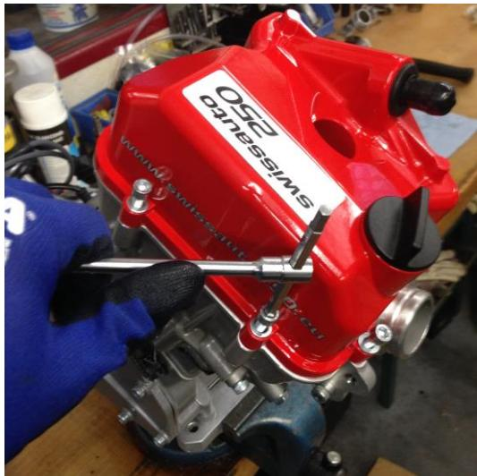
Tighten the 8 M6 bolts by hand.
