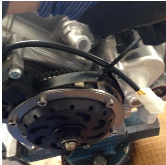
Remove the 1,2mm bended feeler gauge by pulling on the tie-wrap.
