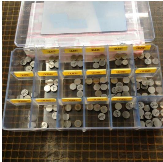
To adjust valve clearance, measure shim, calculate difference and replace with the correct shim. Now the valve clearance is set and ready for later.
