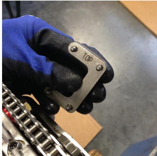
Place the camshaft block tool between the 2 chainwheels. The top is marked on the tool.
