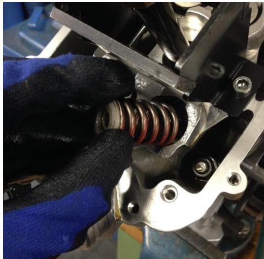
Take off the pressure tool and the valve spring is ready to get out.
