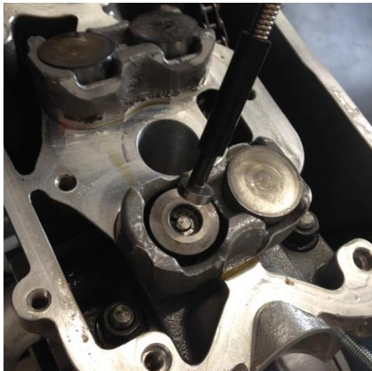
Take off the 4 valve clearance shims; use a magnet to avoid they fall into the engine.
