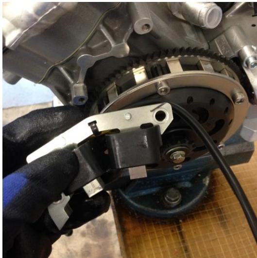
Remove the charge coil (2 M6 bolts).
