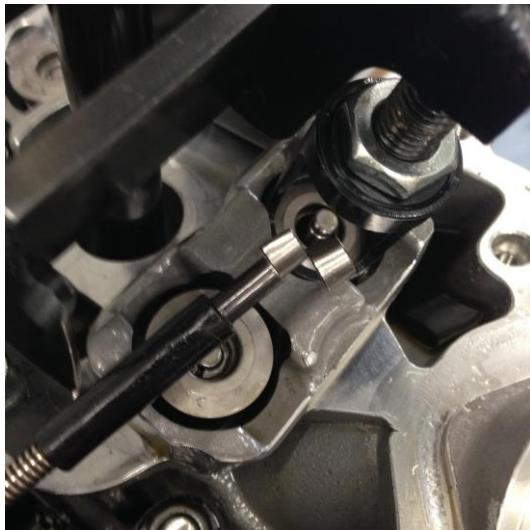
By compressing the valve spring, we create a gap between the retainer and the valve stem keys. Once big enough, it is possible to remove the 2 valve stem keys with a magnet tool.
