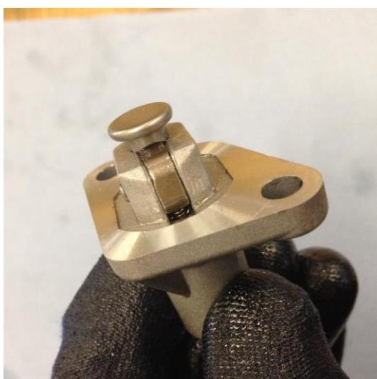
Push the tensioning arm of the automatic cam chain spanner completely to the end. Now it is ready for later.
