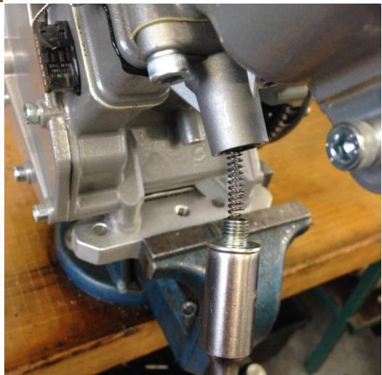
Remove the spring of the automatic cam chain spanner. (1 screw)
