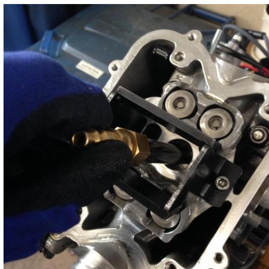
Place the air connector tube in the spark-plug hole.
