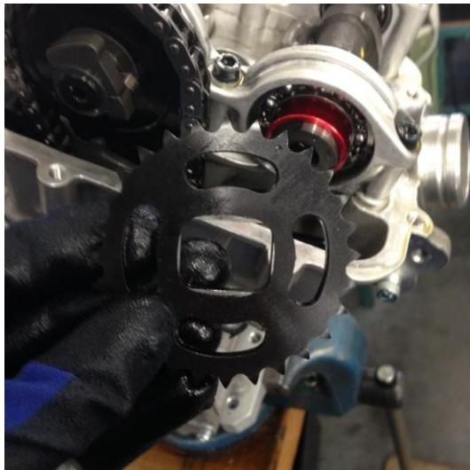
Remove the chain wheel of the inlet camshaft.
