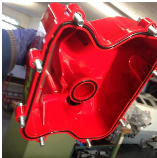
Put on the cam cover. Be sure both O-rings are mount correctly. (If the center rubber is clasped the engine will loose oil trough the 4mm bore above the waterbend on the right side of the cylinderhead.)
