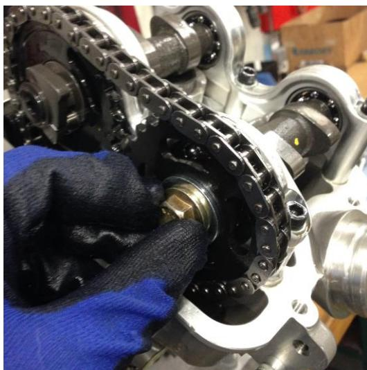
Assemble the M10 bolt and washer on the side of the inlet camshaft. Don't tighten it yet!
