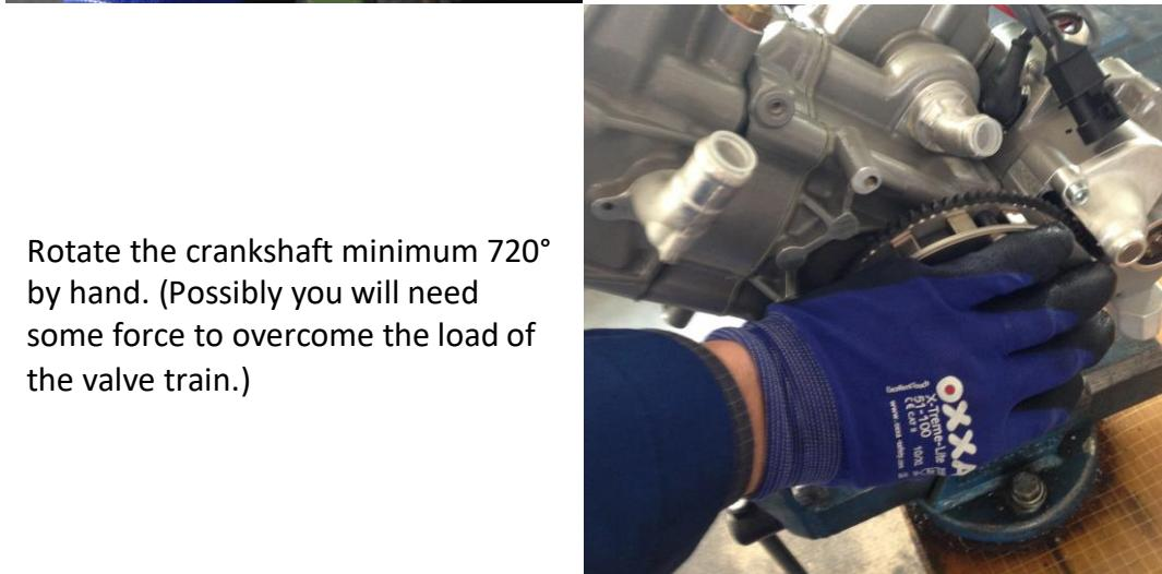
Rotate the crankshaft minimum 720° by hand. (Possibly you will need some force to overcome the load of the valve train.)
