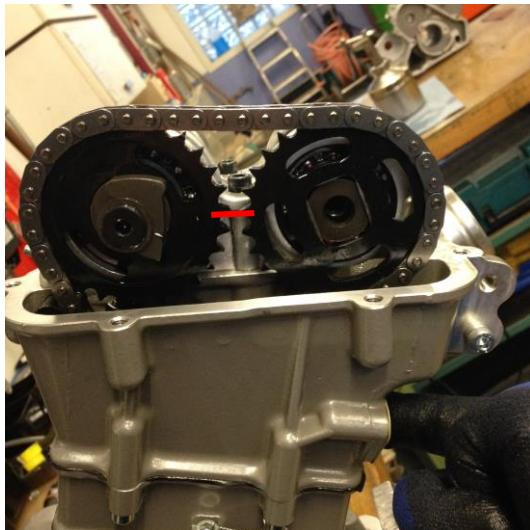
Stick the chain wheel on the inlet camshaft in such way both marks inlet/exhaust point to each other. Push the tension rail with your finger via the opening of the automatic cam chain spanner to get exact position.
