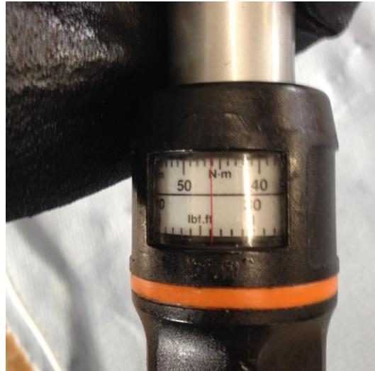
Use a torque wrench to tighten the M10 bolt on the side of the inlet camshaft. Set-up : 46Nm
