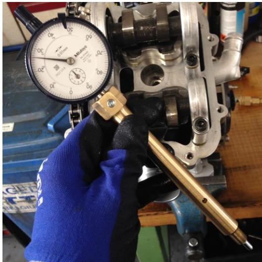
Use the swissauto250 gaging set to put piston in TDC. Screw the gauge into the spark-plug hole and rotate slowly the crankshaft until the piston is in TDC. Zero the gauge!
