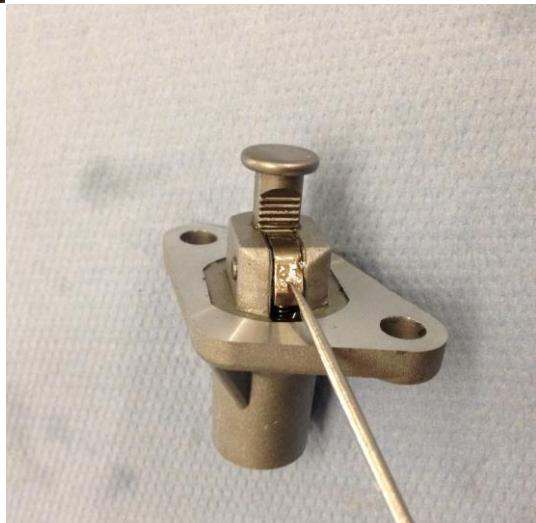
Push down the catch to release the tensioner arm of the automatic cam chain spanner.
