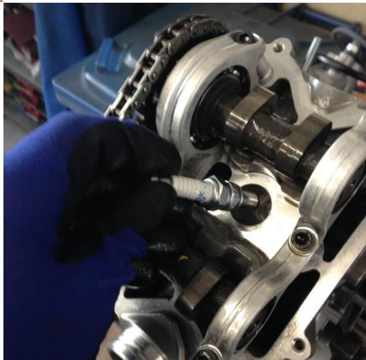
Reinsert the spark-plug and tighten it by hand.
