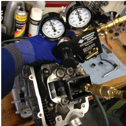
To prevent that the valves drop into the cylinderhead we connect a pressure valve with the air connector tube (maximum 2 bar); in this case we use a leak tester for it.
